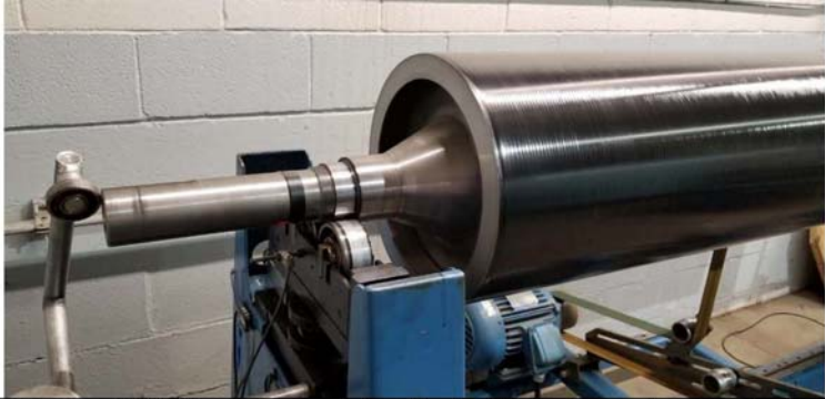
Balancing a 1200 lbf Permanent magnet rotor after ultra-high tension wrapping with carbon fiber
